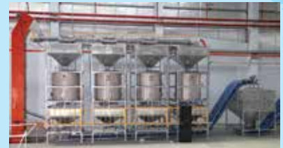
Cashew Steamer Capacity: 800-1,000 kg/Batch
